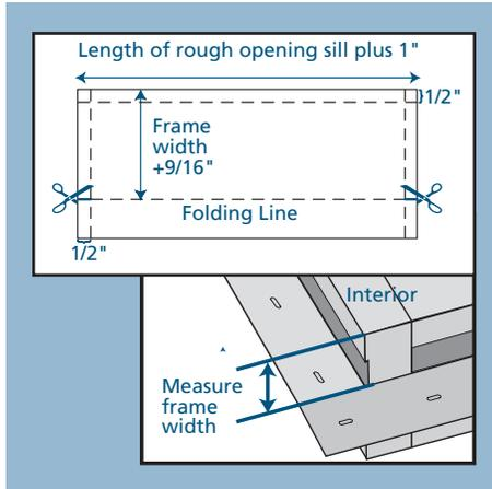
7. Fold the three back sides up to make a 3-sided box, and, for step-down landings, fold the front flap down.
