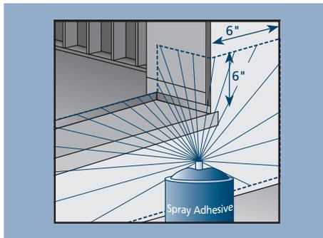
3. Cut a piece of self-adhered flashing the length of the sill and apply over the entire sill pan. For step-down landings, fold flashing down as shown. For continuous slabs, trim flush with rough opening.
