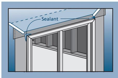
3. Ensure sealant on back dam of the sill pan fully seals to the inside face of the sill. Apply more sealant as necessary.
