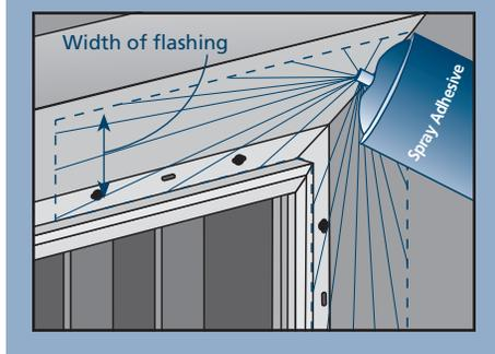
**APPLY THE SELF-ADHERED FLASHING**
