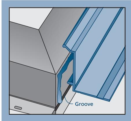
2. Inswing/outswing doors will need a strip of self-adhered flashing applied over the dead bolt hole on the exterior side of the frame as shown.
